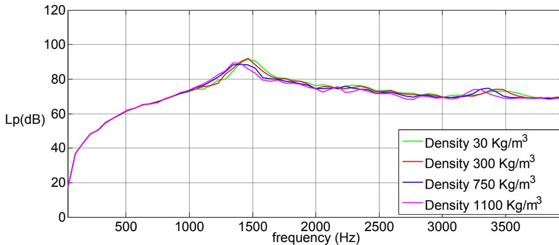
**Figure 11. Parametric analysis, varying only the density of the underlay material.**
