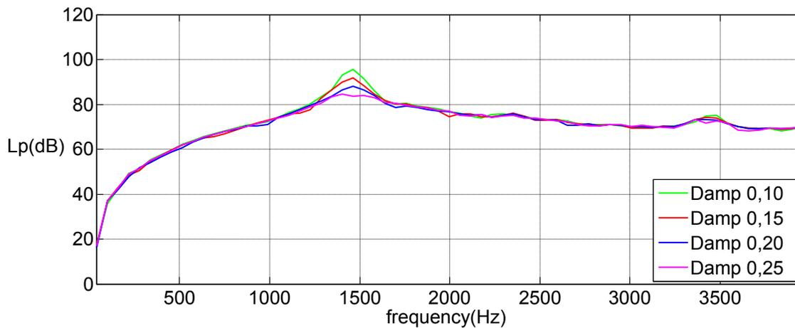
**Figure 12. Parametric analysis, varying only the damping properties of the underlay material.**
