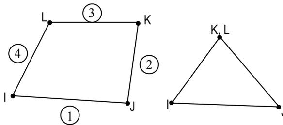
**Figure 6. Element Fluid 29 in its two versions forming quadrilaterals or triangles.**
