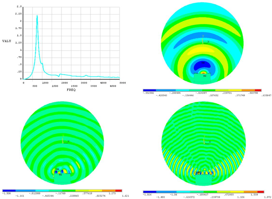
**Figure 9. Distribution of pressure in Pa in the air for 500, 2000 and 4000 Hz, from lower to higher, from a harmonic analysis.**
