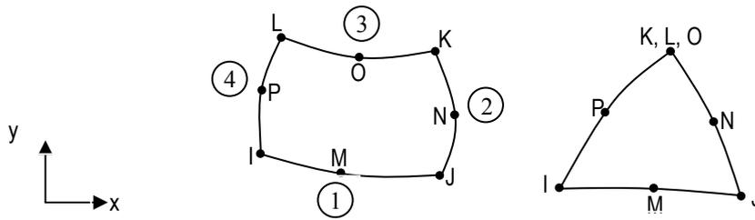
**Figure 5. Element Plane 82 in its two versions forming quadrilaterals or triangles.**
