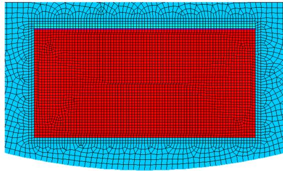
**Figure 8. Mesh of the solid parts of the model simulation, the interface and the surrounding air.**
