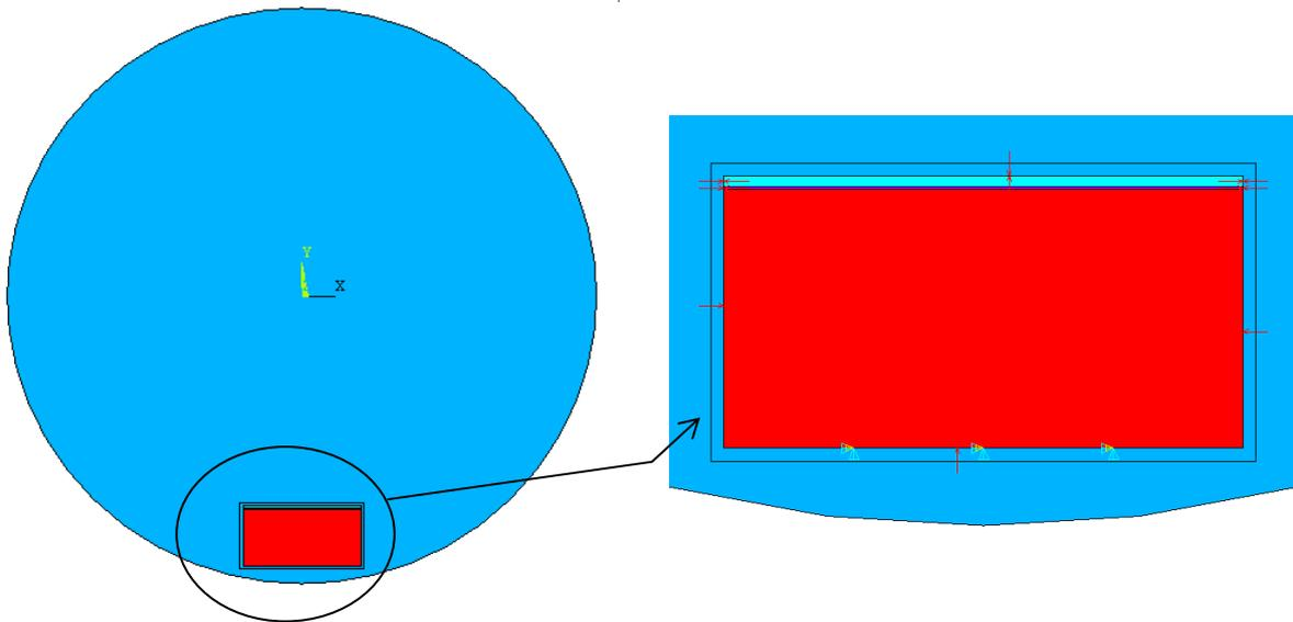
**Figure 3. Model of the complete dimensions, composed of a concrete base, underlay material, laminated floor, air and limit of the solid part to define the fluid-structure interface. The exterior circumference of the circle is of infinite absorption.**
