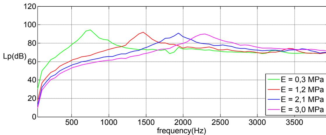
**Figure 10. Parametric analysis varying only the Young model of the underlay material.**
